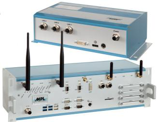
MPL Solutions are modular designed and therefore can be easily expanded and customized to meet various customer needs. The LAN ports come on M12 (D-coded or X-coded). The same applies to the input power. The input power ranges from 9-36VDC, 18-48VDC, or 60-163VDC. The devices can also be equipped with redundant power input. Nearly any additional functions can be integrated over the various expansion buses on the PIP39.
