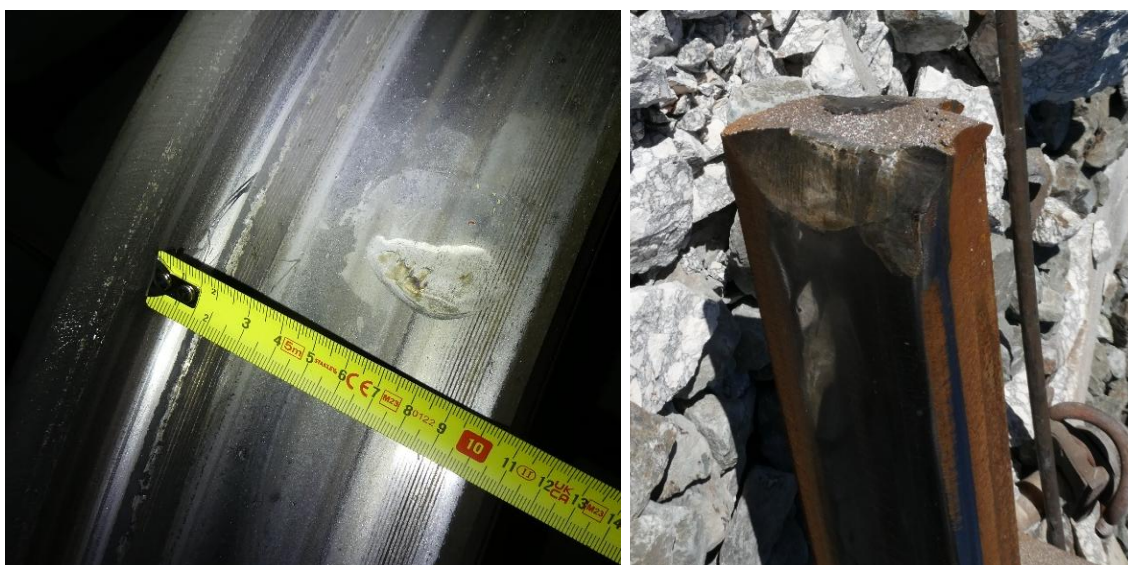
1: Notches found on the right wheel of axle 13 of the Iryo train (4th carriage, first axle of the first bogie) and possible point of collision with the rail head.
