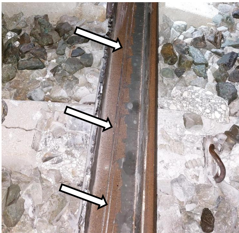
4: Rail lying on its side, after the point of breakage. Traces of the train wheels can be seen on the rail web.
